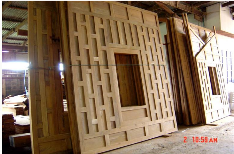
Figure.7 The wall panel ready made from the builder shop.
