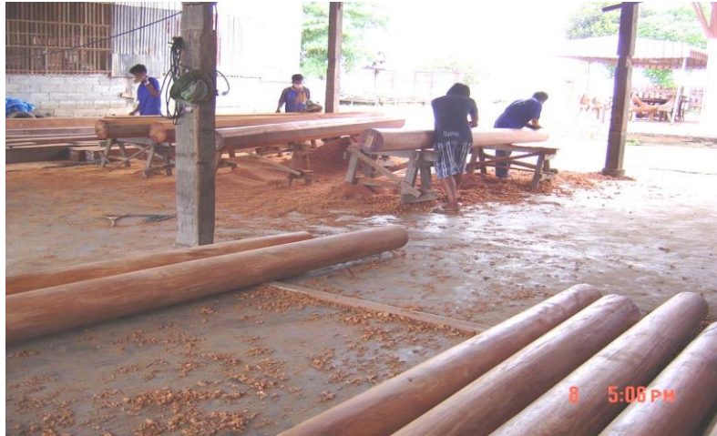
Figure. 10 Skilled craftman worked on teakwood post.
